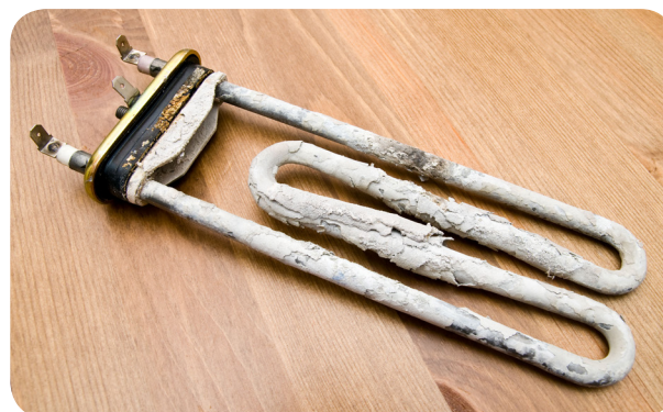
Figure 13.8 Scales on the machine pipes
